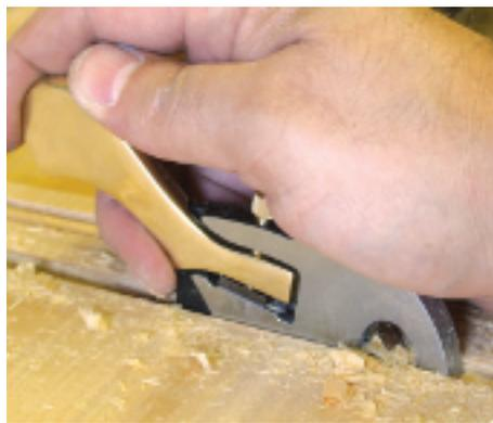
▲ The plane can be used in a variety of ways such as a pull stroke...
