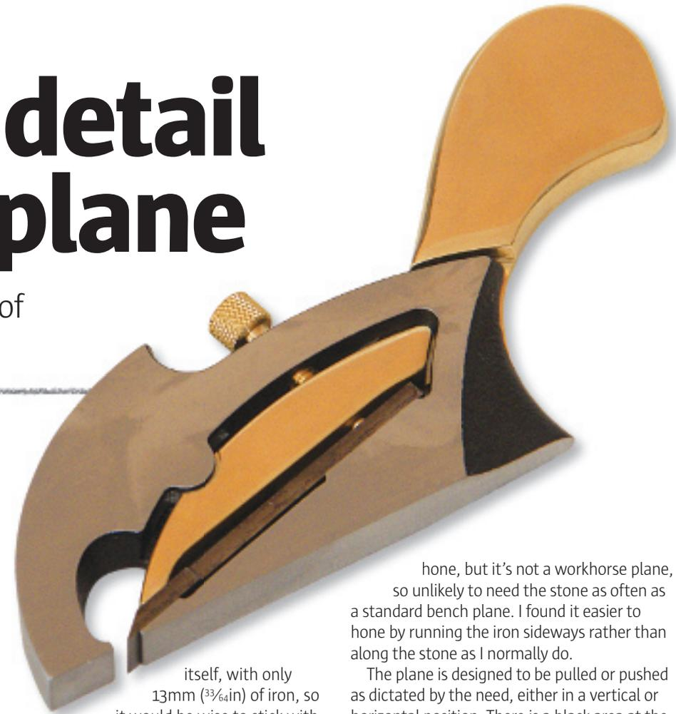
itself, with only 13mm ( $\frac{3}{4}$ in) of iron, so it would be wise to stick with the recommendation of maintaining the primary angle of 30° to prolong the lifespan.
