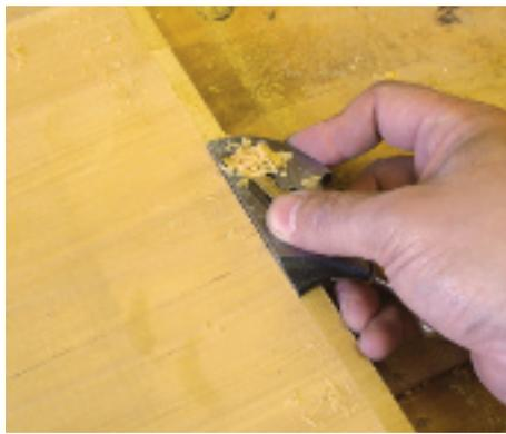
▲ ...or on its side for shoulder trimming on the push stroke
